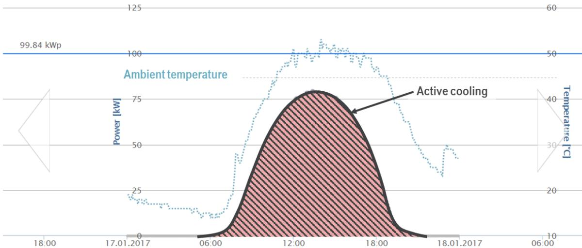
Figure 10: Yield with active cooling [source: Reference system in Australia, Fronius [3] ]
