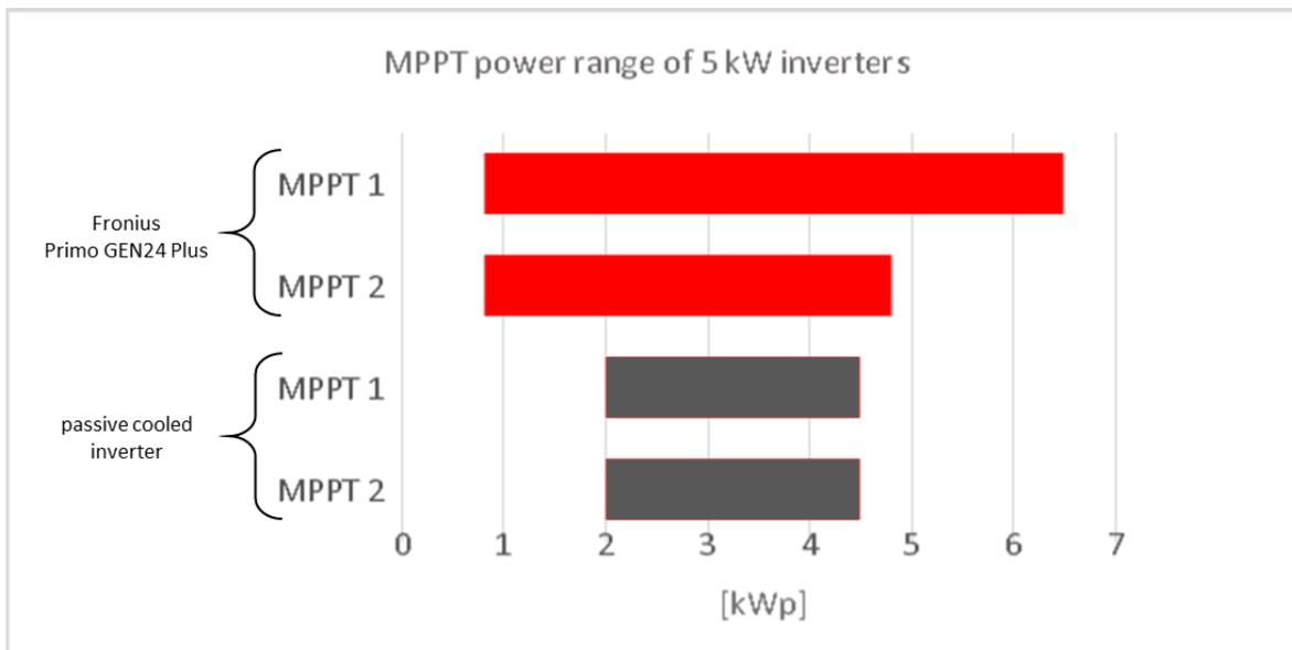
Figure 1: Comparison of MPP tracker power distribution for passively and actively cooled 5 kW inverters
