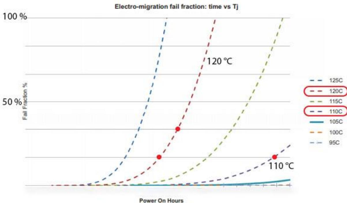
Figure 6: Failure rate subject to temperature and period of operation [source: Texas Instruments [1]]
