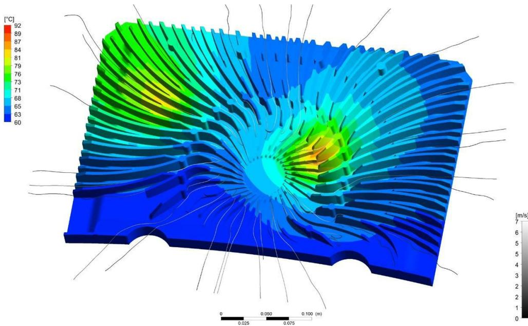
Figure 17: CFD flow simulation – rapid heat removal via the cooling fins [source: Fronius]
