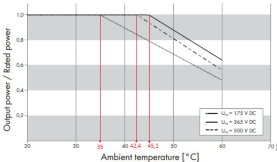
Figure 14: Power derating subject to ambient temperature at PAC,nom = 5 kW [source: competitor data sheet]
