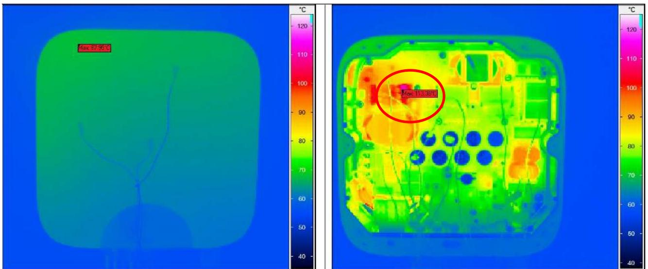
Figure 12: Distribution of heat inside a passively cooled inverter at an ambient temperature of 55 °C (PAC=5 kW,  $U_{mpp}$ =260 V) [source: Fronius]
