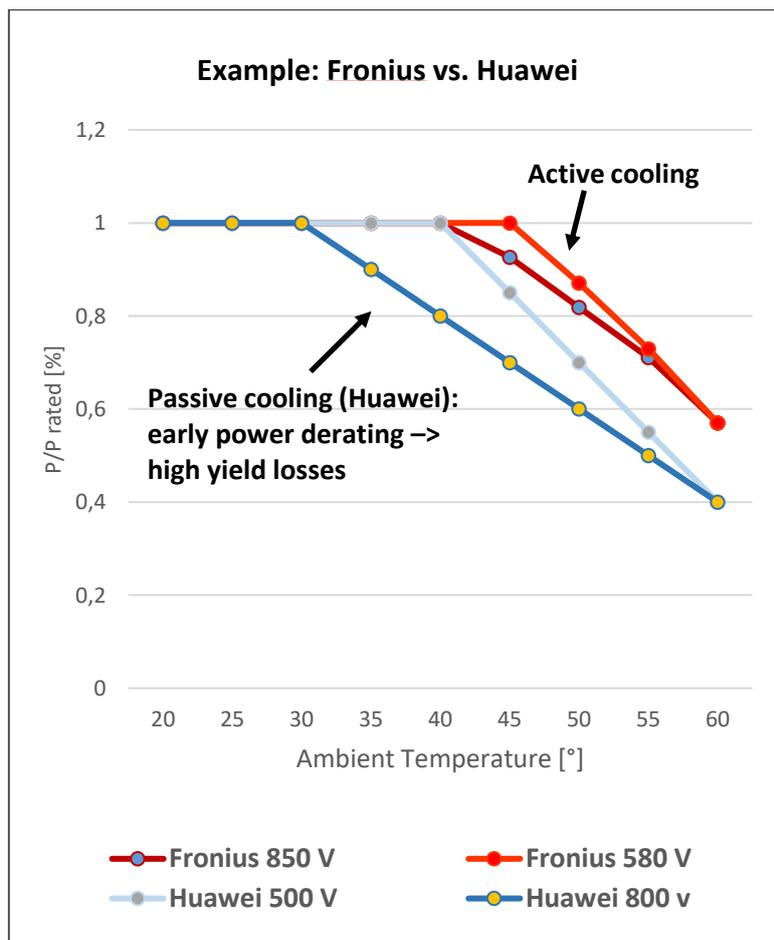
Figure 8: Power reduction in relation to ambient temperature [source: competitor data sheet]
