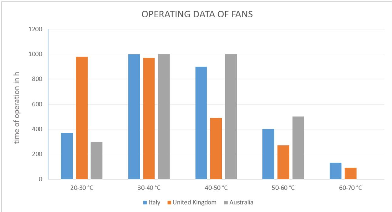
Figure 7: Annual operating data for the fans of actively cooled devices in Australia, Italy and the UK [source: Fronius]
