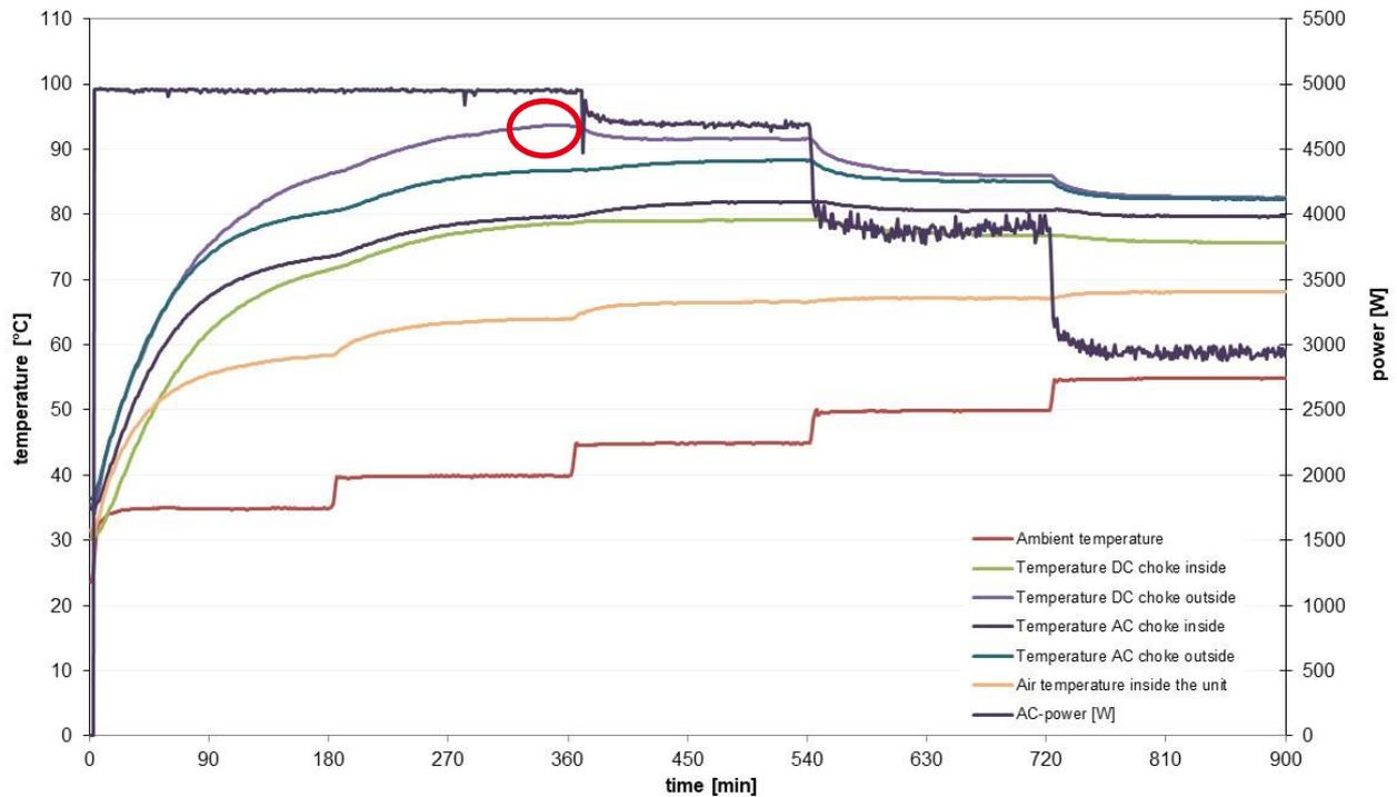
Figure 15: Progression of temperature and power for an actively cooled Fronius inverter (PAC = 5 kW,  $U_{mpp}=220$  V) [source: Fronius measurements]
