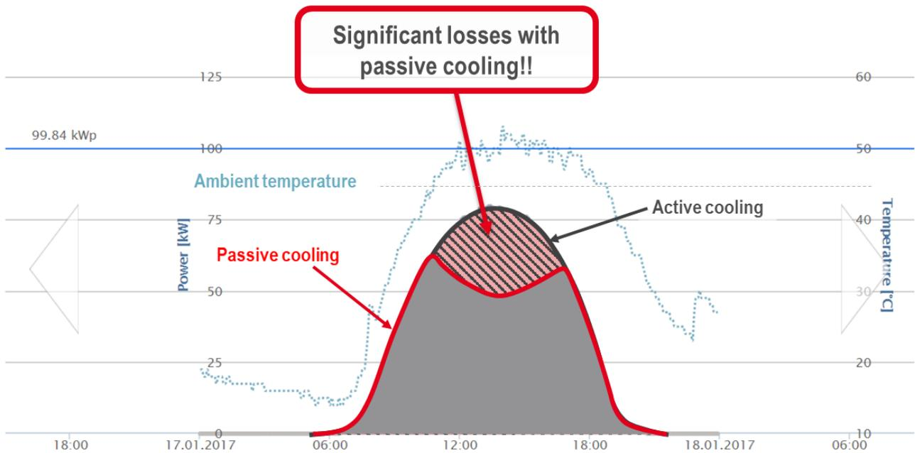
Figure 11: Yield or loss to be expected with passive cooling [source: Reference system in Australia, Fronius [3] ]
