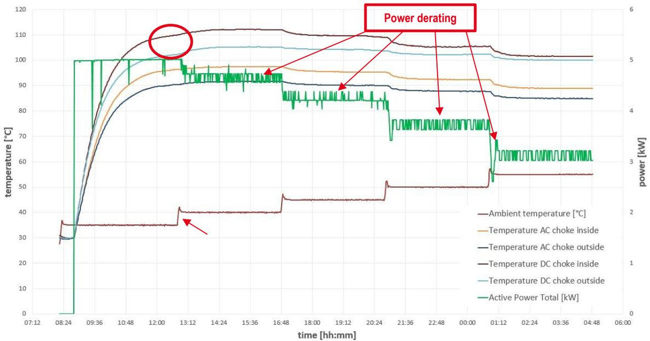
Figure 13: Progression of temperature and power for a passively cooled inverter (PAC = 5 kW,  $U_{mpp,min}=175$  V) [source: Fronius measurements]
