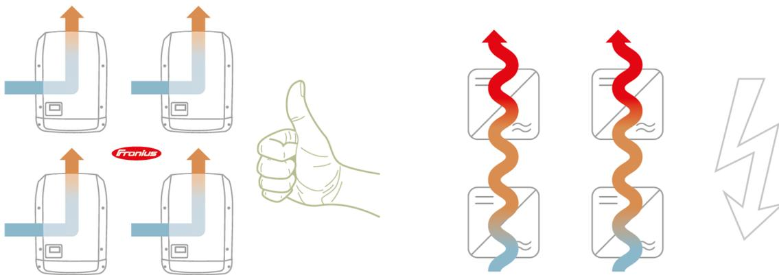
Figure 3: Flexible installation - an intelligent, active air guide allows installation side-by-side or one on top of the other [source: Fronius]
